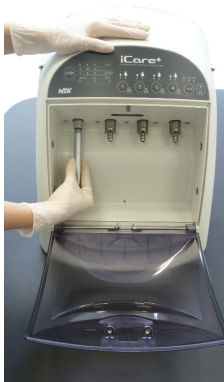
Fig.14 – Connection des turbines
